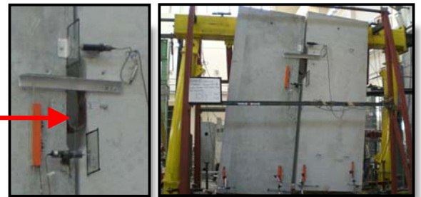
Figure 3: Precast Panels with Steel Cushions (Test II)
