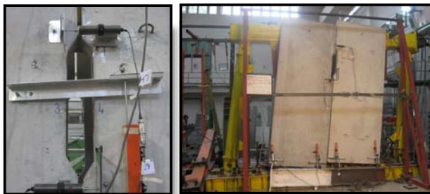
Figure 2: Precast Panels without Steel Cushions (Test I)
