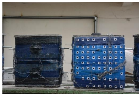
Short column with FRP
