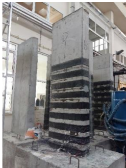
Rectangular RC column with FRP
